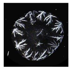
pattern of the water droplets. It can be imaged using a simple digital camera, under side lightening (dark field mode).
