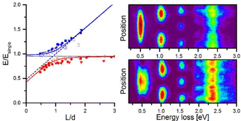
In this research Electron Energy Loss Spectroscopy (EELS) in a Scanning Transmission Electron Microscope (STEM) is applied to probe extraordinary photon transmission through submicron slits in a thin gold film. Coupling of standing-wave-like cavity modes, hybridized with surface plasmon polaritons (SPP), between two adjacent slits, which strongly influences the transmission of light through the slits, is studied by systematically varying the width of the metal bar  $d$  that separates the slits.
