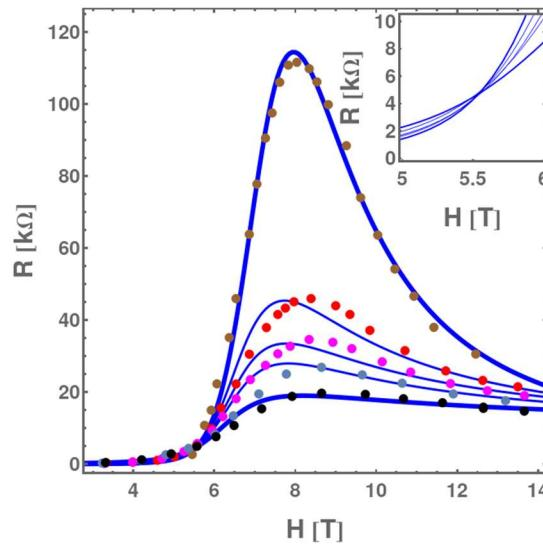
The theory seems also to be applicable to the 2D electron gas formed in the perovskite-oxide SrTiO<sub>3</sub>/LaAlO<sub>3</sub> (111) interface, for which SIT has been observed experimentally under both parallel and perpendicular magnetic fields.
