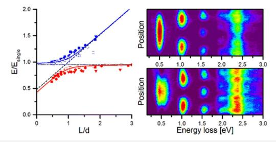
In this research Electron Energy Loss Spectroscopy (EELS) in a Scanning Transmission Electron Microscope (STEM) is applied to probe extraordinary photon transmission through submicron slits in a thin gold film. Coupling of standing-wave-like cavity modes, hybridized with surface plasmon polaritons (SPP), between two adjacent slits, which strongly influences the transmission of light through the slits, is studied by systematically varying the width of the metal bar *d* that separates the slits.
